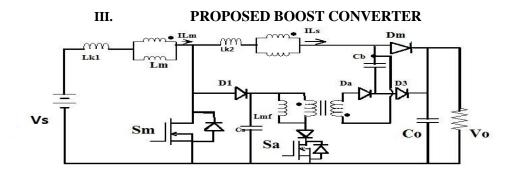
Fig.2: boost converter with snubber and ZVS
