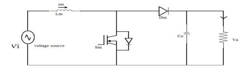
Fig.1: Normal boost converter
